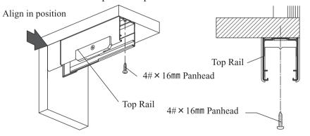
(4) Fit the Top Rail Inner guide to the Top Rail.
