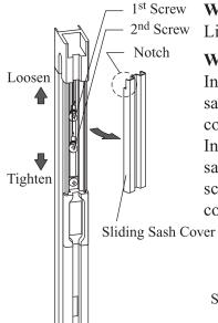
When opening and shutting operation is tight ... Lightly loosen the cord on the 1<sup>st</sup> and 2<sup>nd</sup> screw
