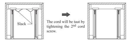
If opening or shutting operation is tight or the Sliding Sash is not parallel, use the following procedure to adjust the cord.
